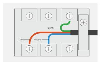
Ensure oven is correctly Earthed and cable clamp is tightened before closing the cover.
